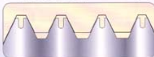
(MIZOBE BOLT joined with nut)
